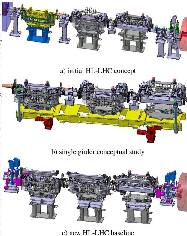
Figure 2: HL-LHC Full Remote Alignment collimator study.
