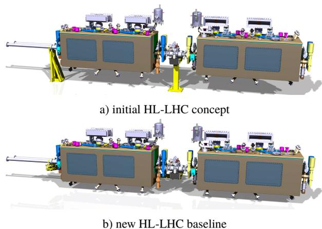
Figure 3: HL-LHC Full Remote Alignment crab cavity study.
