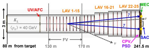
Figure 3: Layout of the detectors for KLEVER.
