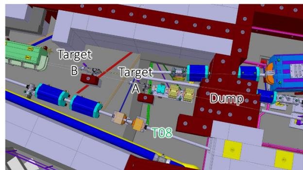
Figure 1: 3D layout of production targets and dump.
