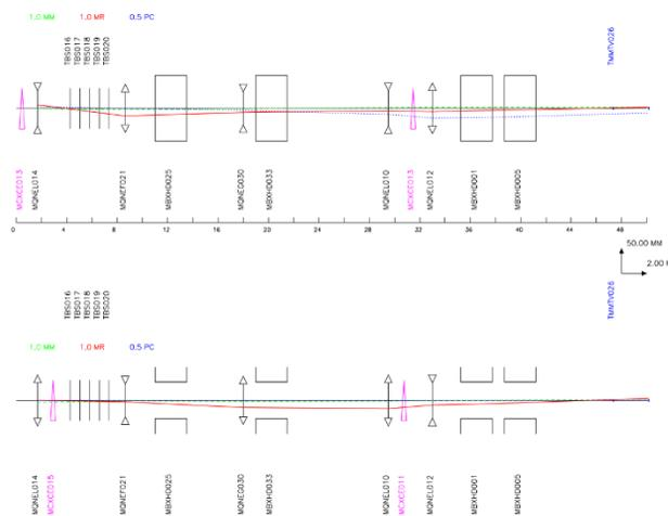
Figure 2: Optics layout of F61 and F62 beam transfer lines. The beam is focused in both planes at the A target (leading to T09 secondary beam line).
