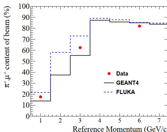
Figure 6: Pion and muon content of the beam in H4-VLE ( $\geq 4$  GeV/c the positron content is not distinguishable in the utilized scheme and therefore added). For momenta  $\leq 3$  GeV/c ( $\geq 4$  GeV/c) the tungsten (copper) target was used.
