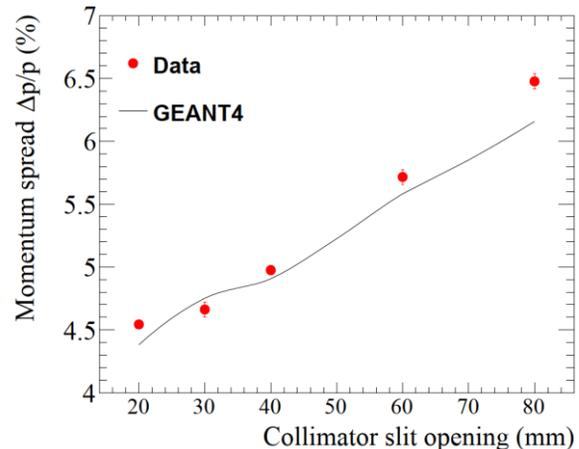
Figure 4: Measured and calculated momentum spread for different slit openings of the momentum-defining collimator and a reference momentum of 7 GeV/c.
