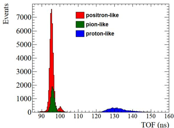
Figure 5: Particle Identification combining time-of-flight measurement and Cherenkov tagging for a 1 GeV/c beam in H4-VLE.
