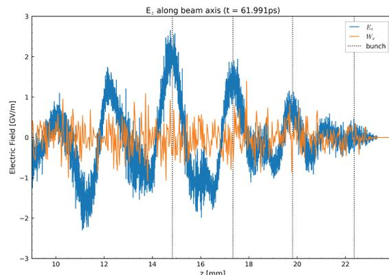
Figure 2: Wakefield simulations using WARP for the 4-bunch train. The centroid locations of the individual bunches are marked by vertical dotted lines, the longitudinal field is given in blue, and the transverse fields in orange.
