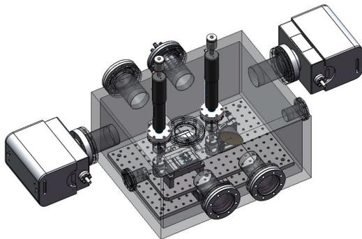
Figure 4: Rendering of experimental chamber and sub-components, including beam diagnostics, laser injection feedthrough, and pumping ports.
