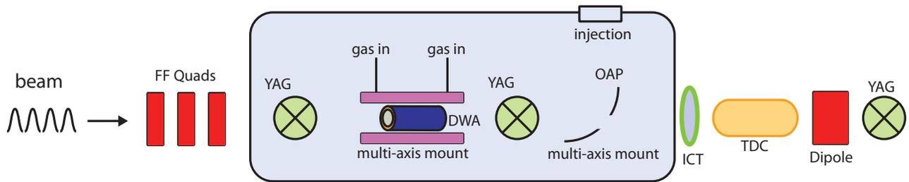
Figure 3: Sketch of the experimental layout. The bunch train is focused through the dielectric capillary using a matching quadrupole triplet. YAG scintillator screens are used for alignment of the beam trajectory to the laser spot. The dielectric structure is mounted on a 5-axis positioner for precision alignment with gas inlets. An off-axis parabolic mirror, with a centered hole, is used to focus the injection laser. Downstream diagnostics include charge and full longitudinal phase space.
