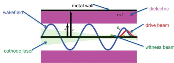
Figure 1: Sketch of dielectric lined waveguide with inner/outer radii  $a/b$ , and injection laser profile in green shadow, drive beam profile in red, and wakefield in blue. The acceleration channel is filled with diffuse gas. Laser ionization occurs at optimal position for trapping and acceleration.
