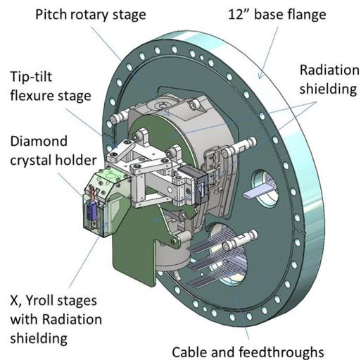
Figure 4: 3D model of the PAL-XFEL self-seeding monochromator 4-axis precision stage system.
