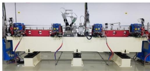
Figure 2: Photograph of the PAL-XFEL self-seeding monochromator integrated on undulator girder system.
