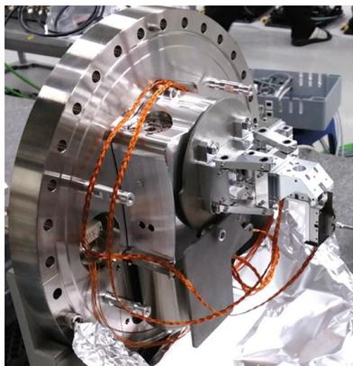
Figure 5: Photograph of the PAL-XFEL self-seeding monochromator 4-axis precision stage system with a dummy of diamond crystals holder for stage test.
