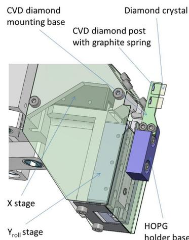
Figure 6: 3D model of the PAL-XFEL self-seeding monochromator thin diamond crystal holder.
