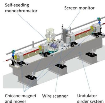
Figure 1: 3D model of the PAL-XFEL self-seeding monochromator integrated on the undulator girder system.
