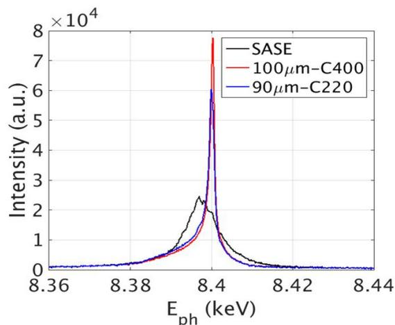
Figure 7: Spectra of the preliminary self-seeding test with PAL-XFEL hard x-ray self-seeding monochromator.
