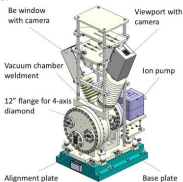
Figure 3: 3D model of the PAL-XFEL self-seeding monochromator UHV enclosure.
