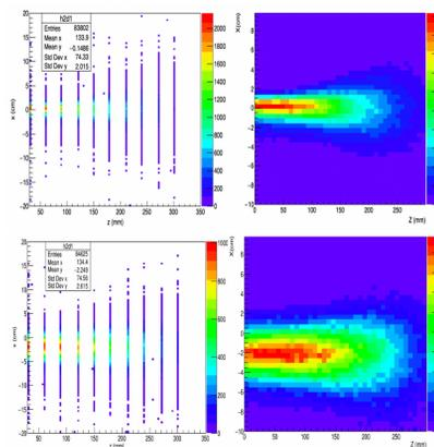
Figure 5: Horizontal beam profile along the longitudinal direction (left) and energy deposition on the  $x$ - $z$  plane (right) in the water box for 70 MeV FLASH beam for Method 1 (top) and Method 2 (bottom).
