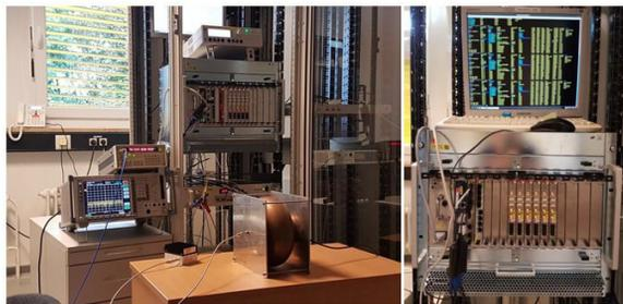
Figure 3: Commissioning and test of the MicroTCA.4-based LLRF system for TARLA.
