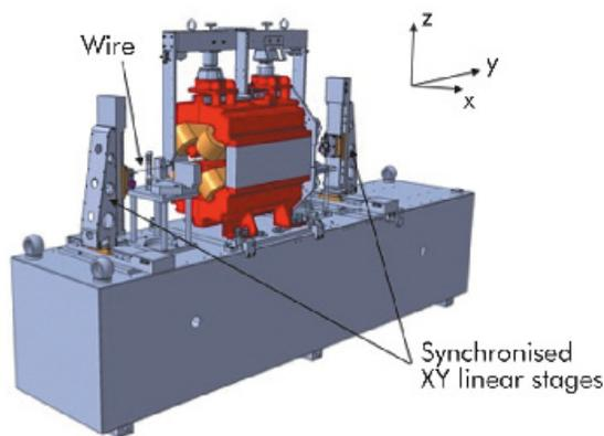
Figure 2: The ESRF stretched wire measurement bench.
