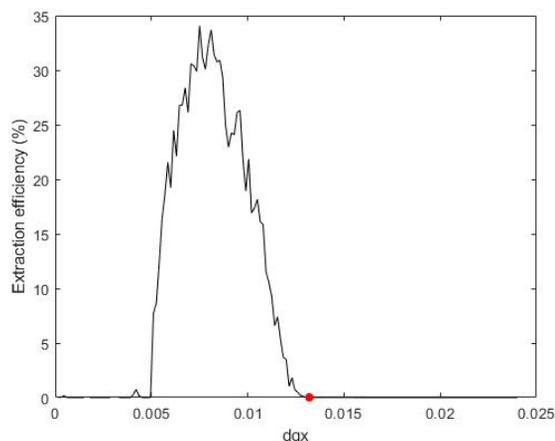
Figure 3: Extracted particles at different machine tunes due only to the effect of the resonance sextupole. Red point indicates the minimum tune that avoids an unwanted extraction.
