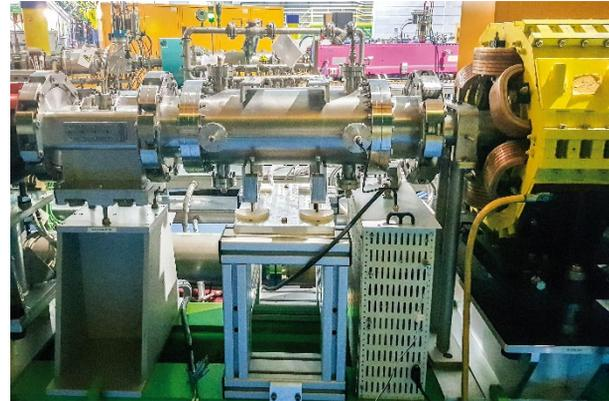
Figure 2: RF-KO kicker installed in CNAO synchrotron.
