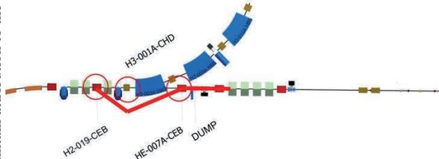
Figure 6: Chopper closure scheme and magnets involved.
