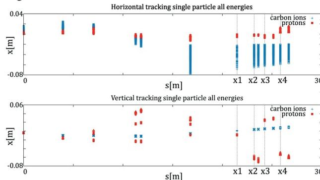
Figure 5: Tracking for both Protons and Carbon ions starting from measured beam position and divergence.
