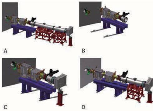
Figure 2: Beamline configurations in the XPR. Scanning magnets and nozzle are mounted on removable supports.
