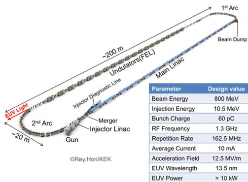
Figure 1: Design and specification of the ERL-FEL light source for EUV lithography.
