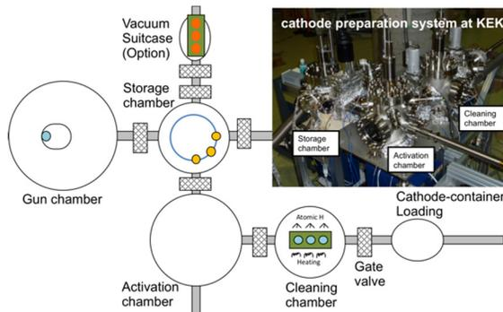
Figure 3: Photocathode preparation system for the DC gun developed at KEK.
