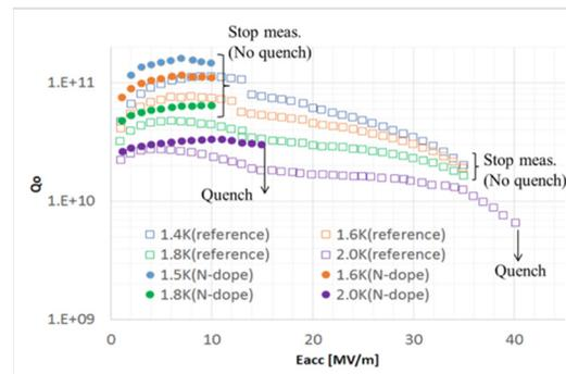
Figure 6: Comparison of Q-values between normal treatment (reference) and N<sub>2</sub> doping treatment.
