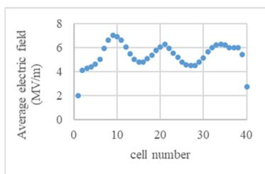
Figure 3: Electric field distribution from 3D simulation.
