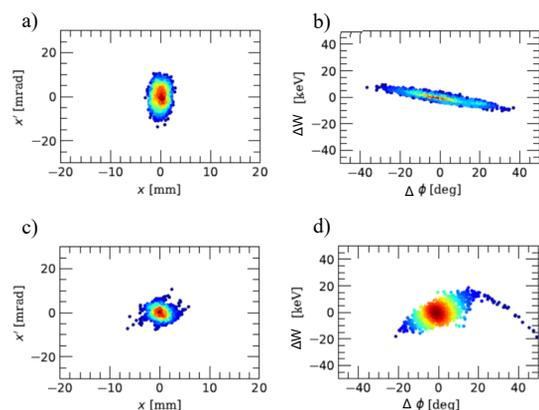
Figure 7: Input and output phase space distributions by MWS and GPT.
