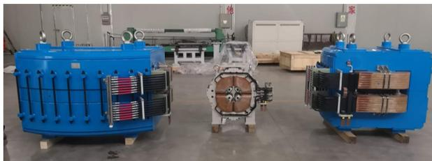
Figure 3: Three prototype magnets, from left to right: (a)  $60^\circ$  dipole; (b) L270 mm quadrupole; (c)  $30^\circ$  dipole.
