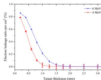
Figure 3: Electron leakage ratio for different target thicknesses.
