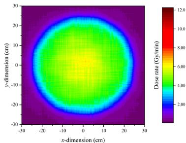
Figure 4: X-ray dose map generated from 2 mm thick target at 4 MeV.
