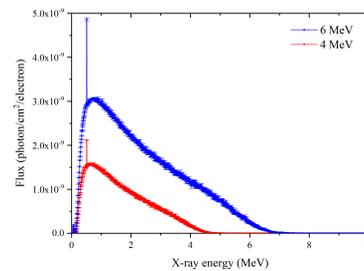
Figure 6: Bremsstrahlung X-ray energy spectra at 4 MeV and 6 MeV.
