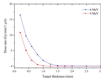
Figure 2: X-ray dose rate for different target thicknesses.
