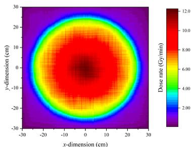
Figure 5: X-ray dose map generated from 2 mm thick target at 6 MeV.
