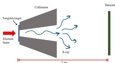
Figure 1: A simple simulation model in FLUKA.
