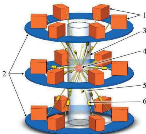
Figure 3: A sketch of the radiographic complex with facilities arrangement in three horizontal planes: 1 – cyclic accelerators; 2 – horizontal planes for accelerators arrangement; 3 – EPC; 4 – test object; 5 – shadow image recording system; 6 – X-ray collimation system.
