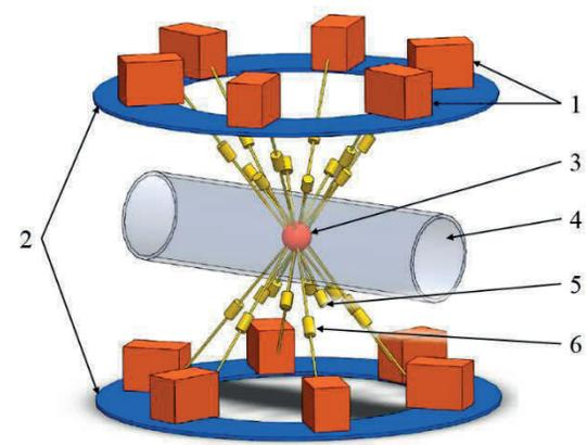
Figure 2: The sketch of a radiographic complex with a horizontal arrangement of the EPC: 1 – cyclic accelerators; 2 – horizontal planes for accelerators arrangement; 3 – test object; 4 – EPC; 5 – shadow image recording system; 6 – X-ray collimation system.
