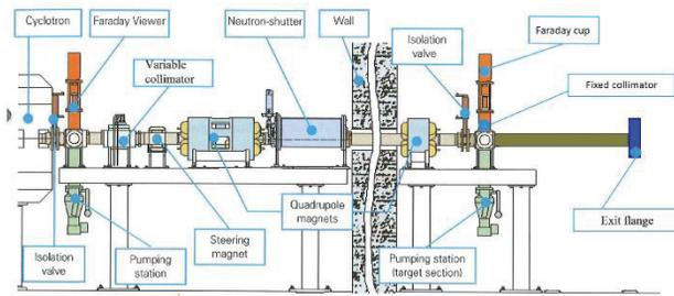
Figure 3: Layout of the external beam line.
