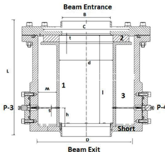
Figure 1: Dielectric-filled re-entrant cavity resonator as beam current monitor. The pickups in the figure represent the large magnetic loops in one plane (as port 3 and 5). Two small magnetic loops are in the other plane (as port 4 and 6). Port 1 is the beam entrance and Port 2 is the exit [3].
