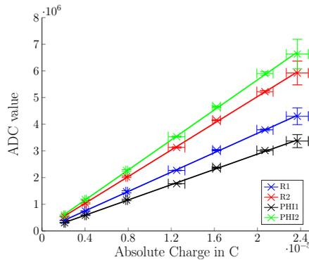
Figure 4: Beam current measurement with a 7 mm collimator. R1 and PHI1 corresponds to the R- and Phi-sensor of module 1, R2 and PHI2 to module 2.
