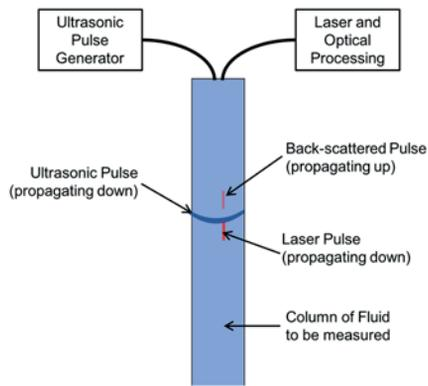
Figure 2: Representation of ultrasonic pulse and delayed laser pulse interacting in fluid column. The laser pulse is scattered upward and shifted in frequency.
