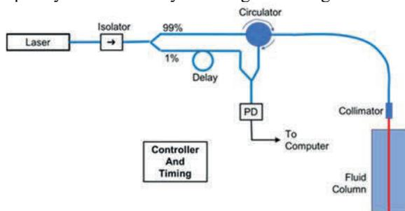
Figure 3: Laser and optical processing elements (not all elements are shown).
