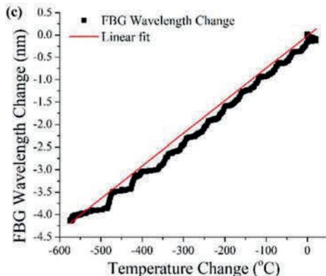
Figure 5: Result from [4] showing nearly linear relation between wavelength shift and temperature change in liquid.
