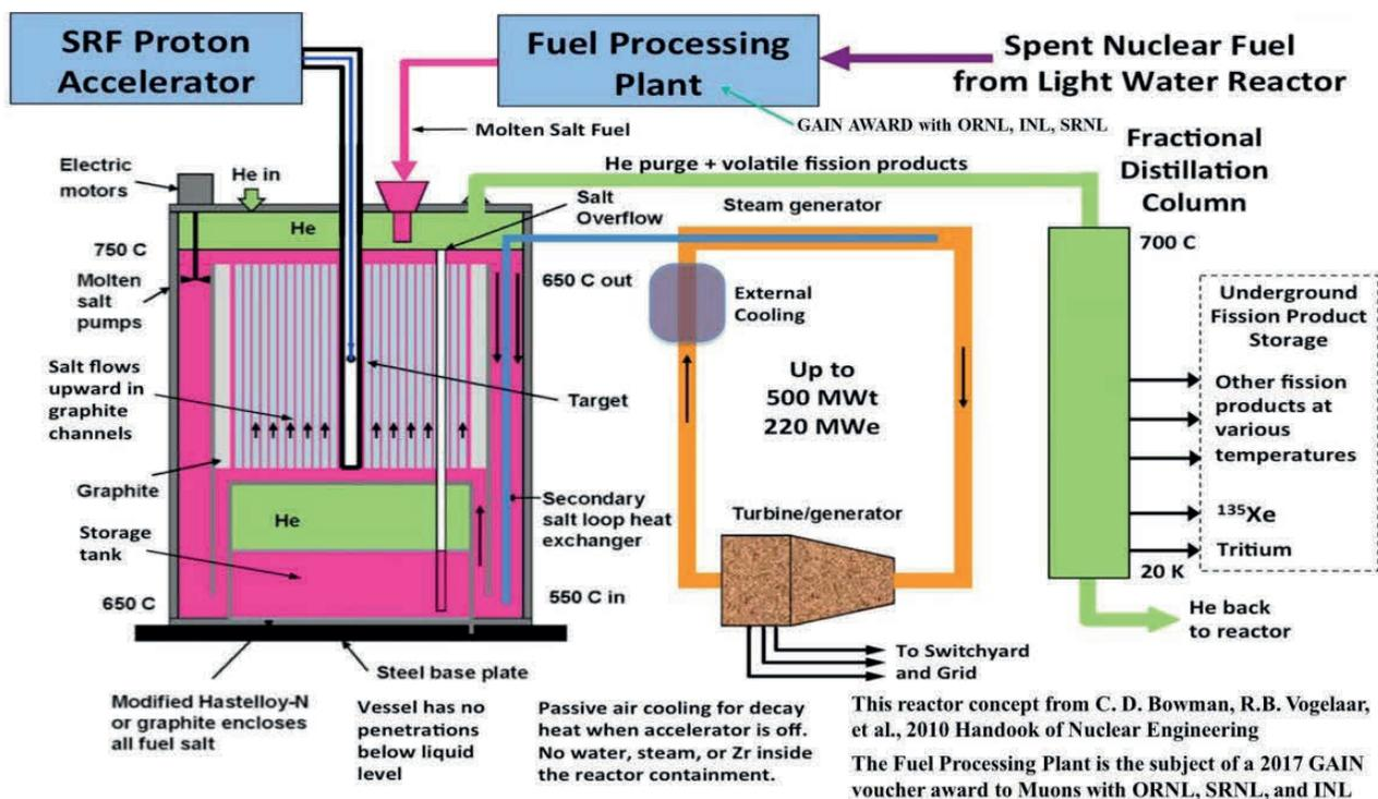
Figure 1: Mu\*STAR reactor system. The reactor core, shown at left, is made of graphite cylinders filled with molten salt that circulates upward through the cylinders. Measurement of the temperature distribution in the various cylinders is an intended application of the method presented in this paper.
