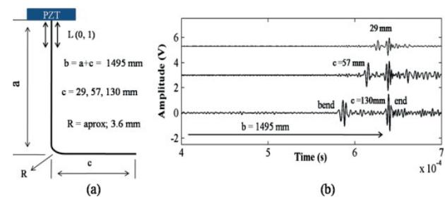
Figure 4: Results from Reference [3] method for sending and receiving an acoustical pulse using a solid waveguide, bent at several places. The time difference between the pulse reflected at the bend and that reflected at the end depends on the temperature along the waveguide.
