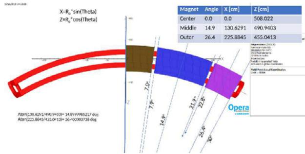
Figure 4: iRCMS sector layout, from the STEP file geometry, as used in OPERA magnet computation.
