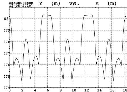
Figure 5: Scalping of the reference trajectory, along the 18.25 m long 180° arc.
