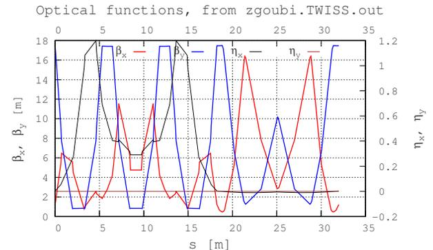
Figure 6: Optical functions from the ‘DIPOLE’ model. It can be observed that the 180° arc comes out quasi achromatic as expected.
