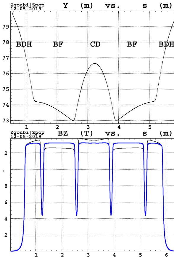
Figure 7: Top:  $\approx 0.7$  cm scalloping of the reference orbit, along the 60° WM field map sector. Bottom: field along the R=508.022 cm arc (blue) and along the scalloping reference orbit (red).
