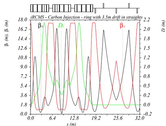
Figure 3: Optical functions in iRCMS half-ring, in the MADX model. These quantities are taken as the design goals, in particular the  $180^\circ$  arc is an achromat.
