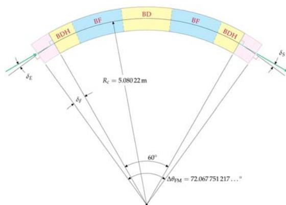
Figure 2: Geometry of the iRCMS BDH-BF-BD-BF-BDH  $60^\circ$  sector OPERA field map, with angular extent  $\Delta\theta_{FM}$ . A reference arc is defined at  $R = 508.022$  cm.  $\delta_F = (\Delta\theta_{FM} - 60)/2$  degree is an additional (entrance and exit) extent that accounts for BDH field fall-offs.  $\delta_E = -\delta_S (= -\delta_F)$  are the angles that the reference orbit makes with the sector at respectively entrance into and exit from the field map.
