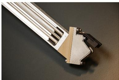
Figure 8: Ion-12SC internal liquid target with aluminum window.
