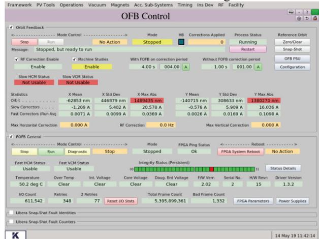
Figure 3: Main Orbit Feedback Control Screen.
