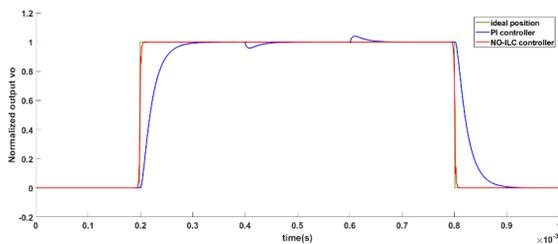
Figure 2: Comparison of system performance for PI and NO-ILC after 30 iterations.
