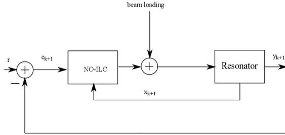
Figure 1: Block diagram of norm-optimal ILC.
