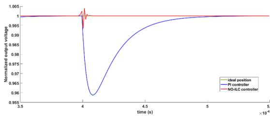
Figure 3: Comparison of beam loading compensation for PI and NO-ILC after 30 iterations.
