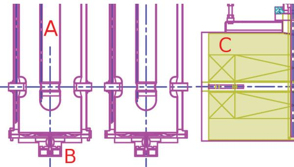
Figure 1: Reference drawing, showing half of a 4 resonator SCB-type module and half the central focusing solenoid. The cryomodule is mirror symmetric about the right edge of the drawing. Labels denote: (A) central resonator, (B) grounded outer resonator surface and (C) solenoid. Beam runs from left to right.
