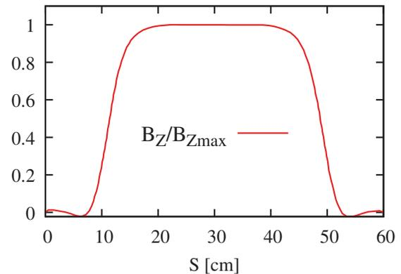
Figure 3: Mapping of the SCB cryomodule magnetic field z-component, as supplied to TRANSOPTR.
