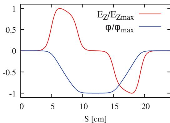
Figure 2: Opera-2D computed potential ( $\phi$ , blue) and on-axis electric field (red) for an SCB cryomodule.
