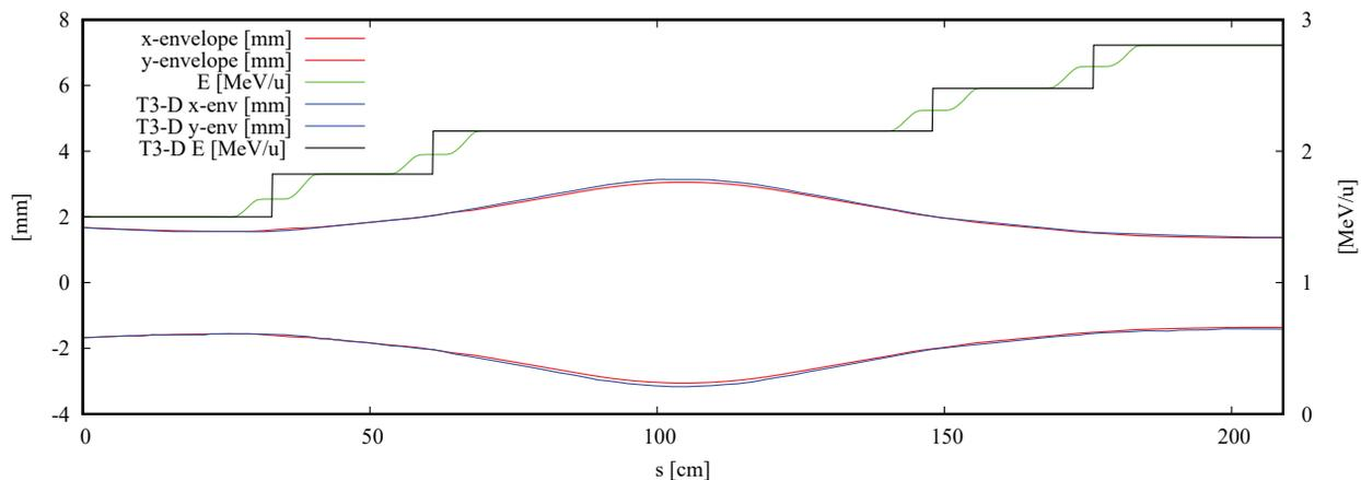
Figure 4: Transverse beam envelope and energy/nucleon for a beam 30 amu, charge state 10, and input velocity  $\beta = 0.057$  calculated using both the Trace-3D and TRANSOPTR models. The transverse envelopes defining the 2RMS contours of the beam distribution (left y-axis), in addition to the energy (right y-axis) are presented for a generic SCB cryomodule.
