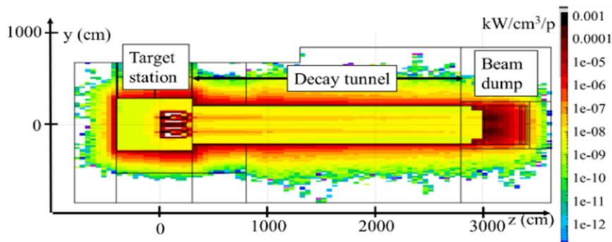
Figure 3: Power density deposited in the whole system.
