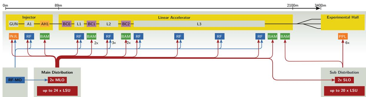
Figure 1: Layout of the pulsed optical synchronization system of the European XFEL. Stabilized fiber links, MLO/SLO and FSD are presented in red. The RF reference distribution system including the RF-MO and the REFM-OPTs is shown in blue. BAMs are illustrated in green and external laser systems in orange.
