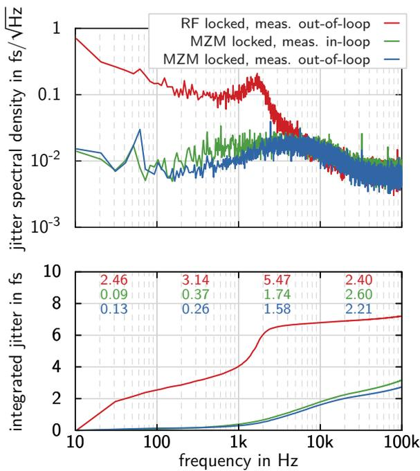
Figure 2: Short term performance of the MLO PLL. A significant improvement has been achieved by implementing an MZM-based laser-to-RF phase detector. The out-of-loop measurements confirm the result.
