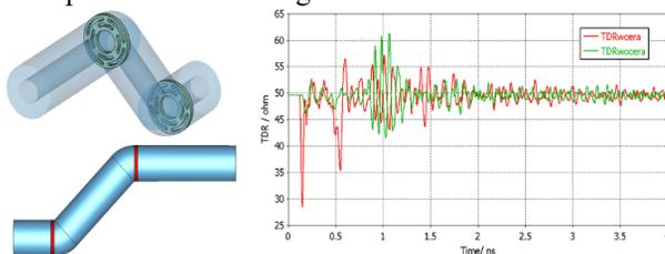
Figure 4: Simulation result of coaxial bend transition part.
