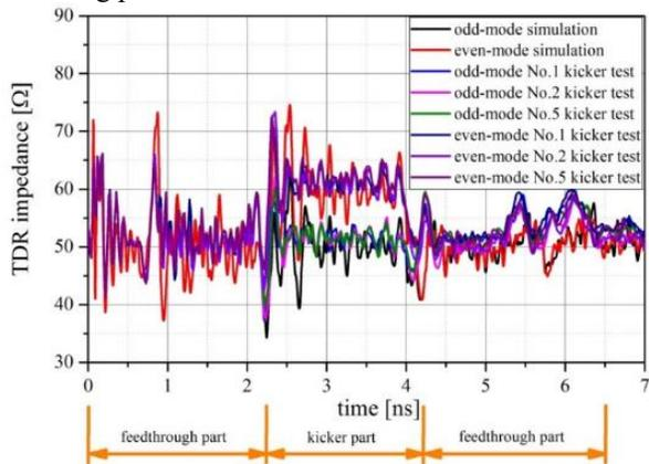
Figure 10: Time-domain reflectometer of prototype kicker.
