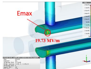
Figure 5: Maximum local electric field intensity distribution.
