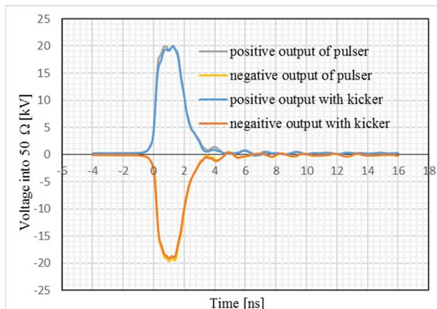
Figure 12: The HV test pulse waveform.
