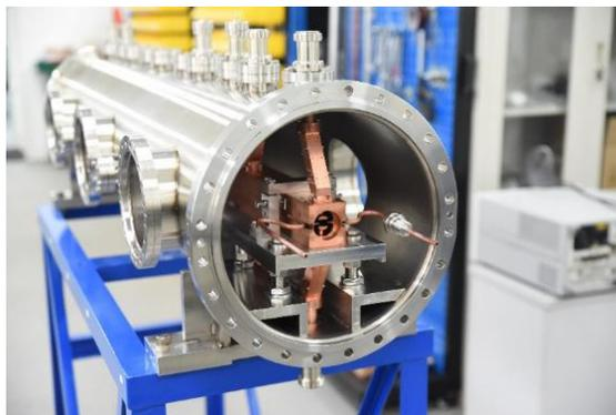
Figure 9: The final assembly of the prototype kicker.
