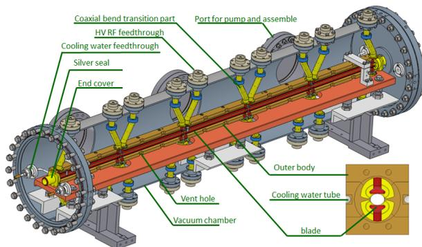
Figure 3: 3D mechanical assembly drawing of kickers.
