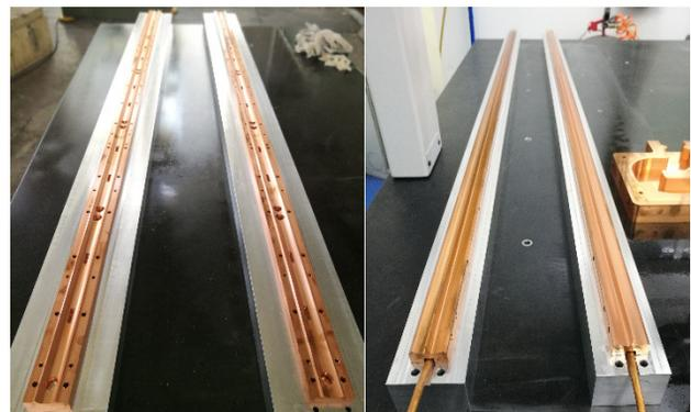
Figure 6: Outer body of strip-line kickers.
