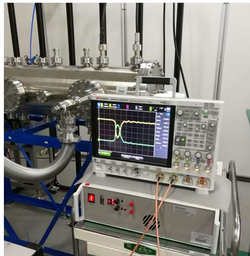
Figure 11: The prototype kicker HV test setup.
