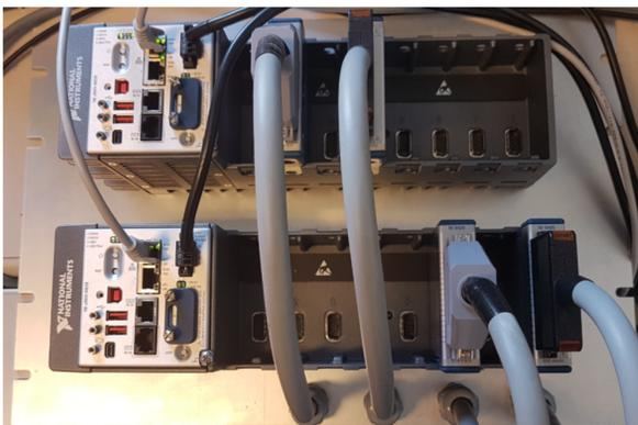
Figure 5: The two National Instruments cRIO-9039 running the same FPGA code in dual modular redundancy mode.
