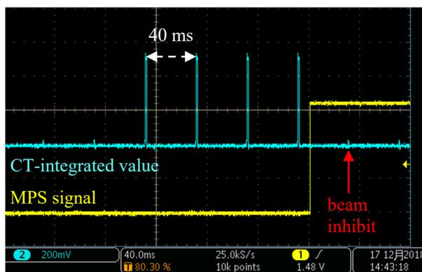
Figure 6: Result of performance test for function (2). (case of beam repetition at 25 Hz).
