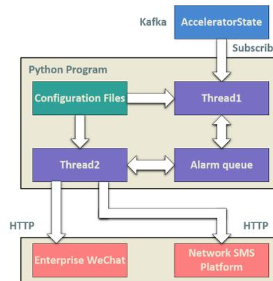
Figure 4: Architecture of WeChat and SMS messages distributors.
