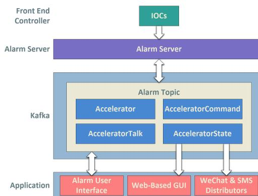
Figure 1: Architecture of the IRFEL alarm system.
