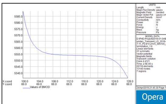
Figure 4: Main field transverse homogeneity in X direction.
