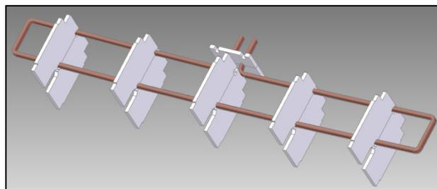
Figure 10: Coil support structure of the thin septum.
