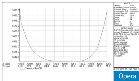
Figure 5: Main field transverse homogeneity in Y direction.
