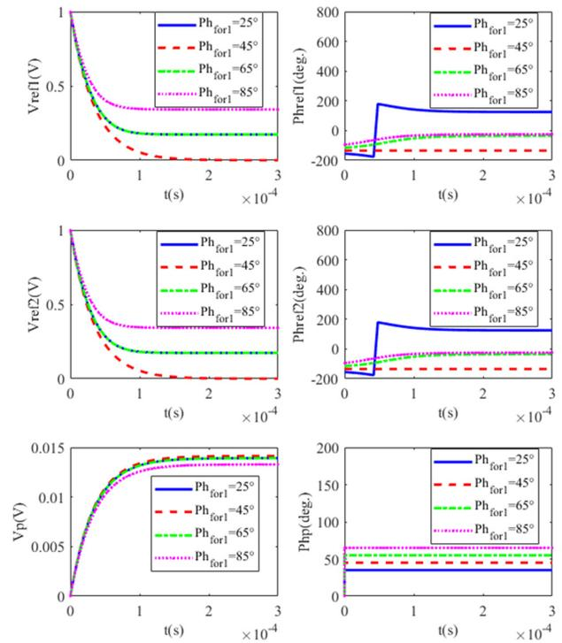
Figure 5: The amplitude and phase of  $\tilde{V}_{ref1}$ ,  $\tilde{V}_{ref2}$  and  $\tilde{V}_p$  in different phases of  $\tilde{V}_{for1}$ .
