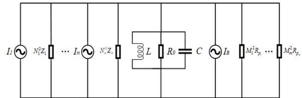
Figure 2: Equivalent parallel LCR circuit of multi-feeding cavity with beam loading at cavity side.
