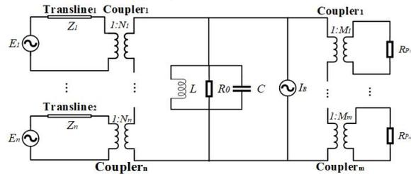
Figure 1: Equivalent circuit LCR model of multi-feeding cavity with beam loading.
