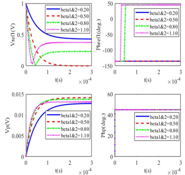
Figure 3: The amplitude and phase of  $\vec{V}'_{ref1}$ ,  $\vec{V}'_{ref2}$  and  $\vec{V}'_P$  in different  $\beta_1$  and  $\beta_2$ .
