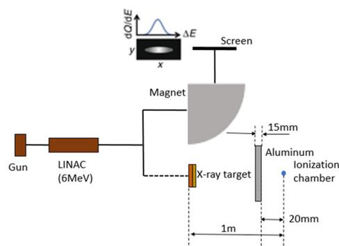
Figure 3: Schematic of dose measurement experiment.
