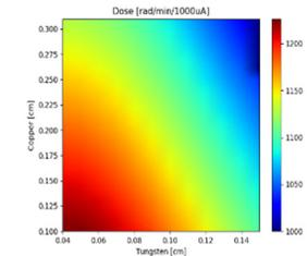
Figure 2: Dose rate of tungsten-copper target.
