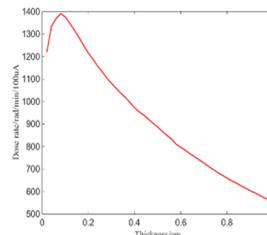
Figure 1: Dose rate of single tungsten target.
