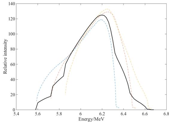
Figure 4: Electron energy spectrum at 10 KV gun voltage.
