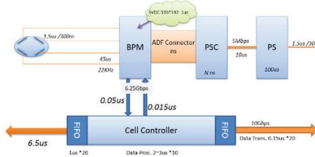
Figure 6: Preliminary time consumption estimation in each step.
