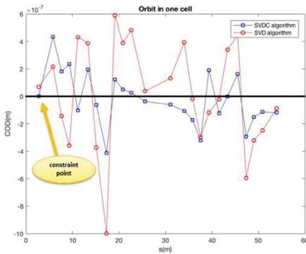
Figure 2. The orbit after correction in one period.
