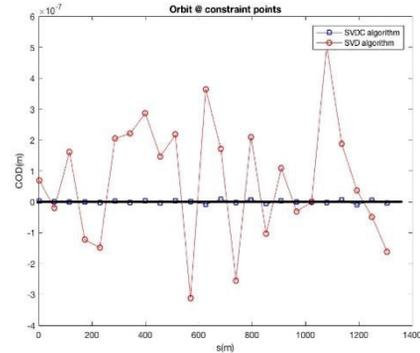
Figure 3: Comparison between the SVDC and SVD algorithm at the constraint points (the first BPM in each cell) around the ring. The SVDC can suppress the closed orbit distortion effectively at specific places.
