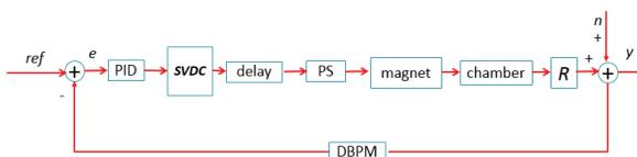
Figure 7: Feedback loop of fast orbit feedback system with SVDC.
