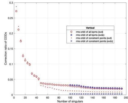
Figure 4: Results comparison of SVDC and SVD, SVDC algorithm can help suppress the orbit at constraint points.
