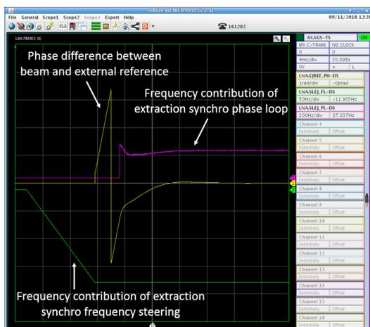
Figure 3: Extraction synchronisation process for an antiproton beam at  $h = 4$  and a reference at  $h = 1$ .
