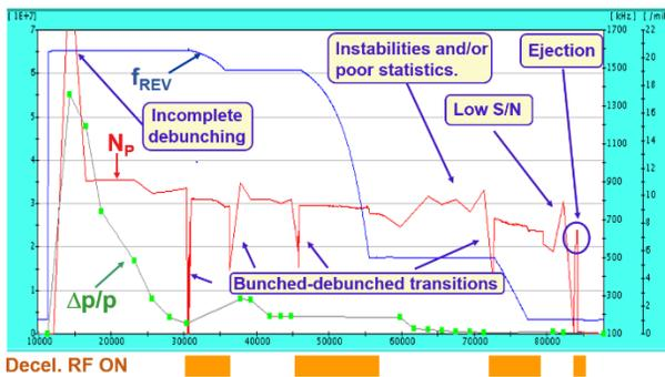
Figure 5: Longitudinal diagnostics plot for an AD cycle.
