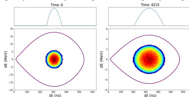
Figure 3: Phase space simulation for the first ramp beginning (left) and end (right).
