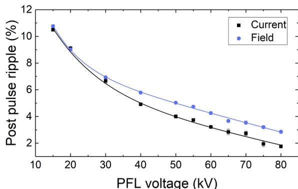
Figure 7: Post-pulse ripple amplitude evolution with respect to PFL voltage for current (black) and magnetic field (blue).
