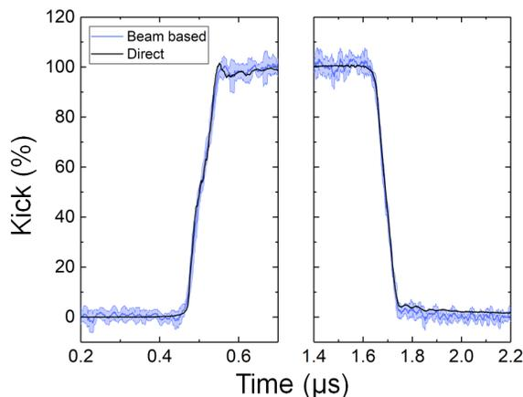
Figure 5: Rise and fall times comparison of beam based (BB) measurement (blue) and direct measurements (black).
