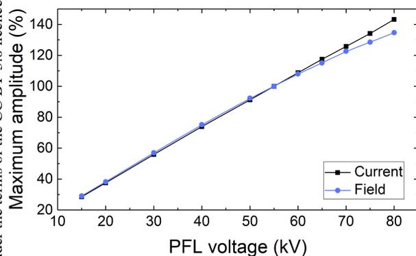
Figure 8: Flap-top kick amplitude with respect to the PFL voltage for current (black) and magnetic field (blue).
