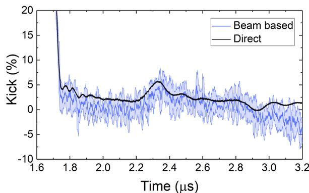
Figure 6: Post-pulse comparison of beam based (BB) measurements and direct measurements (back).
