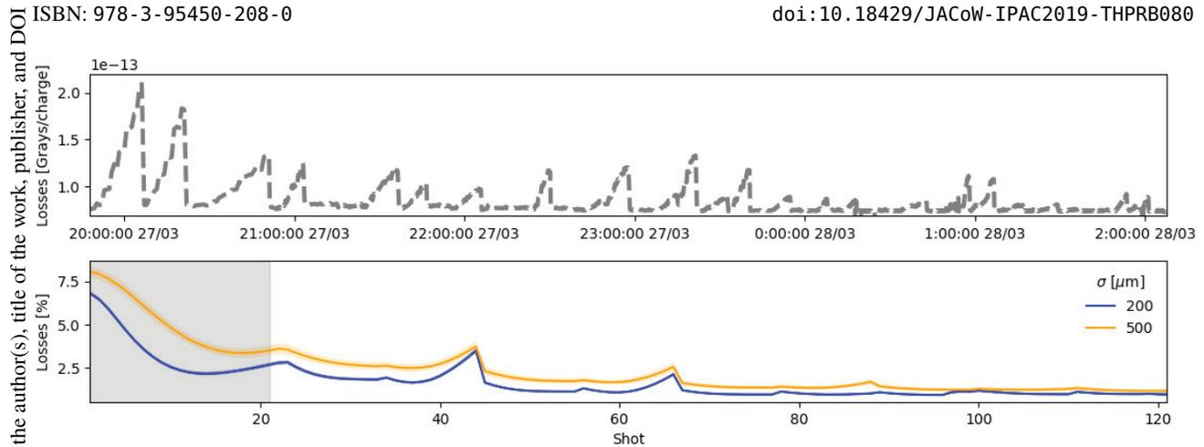
Figure 1: Top: Normalised BLM losses measured over 6 h for a single alignment session during 2018 re-commissioning. Overall improvement was 31%. Bottom: 500 anode scan simulations with normally distributed initial misalignments. Average and 95% confidence interval of the losses is shown. Shaded area indicates girder scan with subsequent scans following ZS tank anodes 1 to 5.
