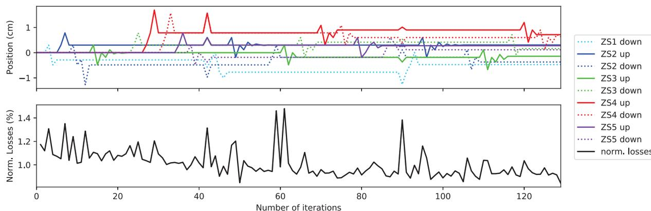
Figure 3: Beam test of automated alignment using Powell's method. The anodes were set to zero to simulate a restarting scenario. The algorithm was stopped after 129 iterations, where the losses were reduced by more than 28 %.
