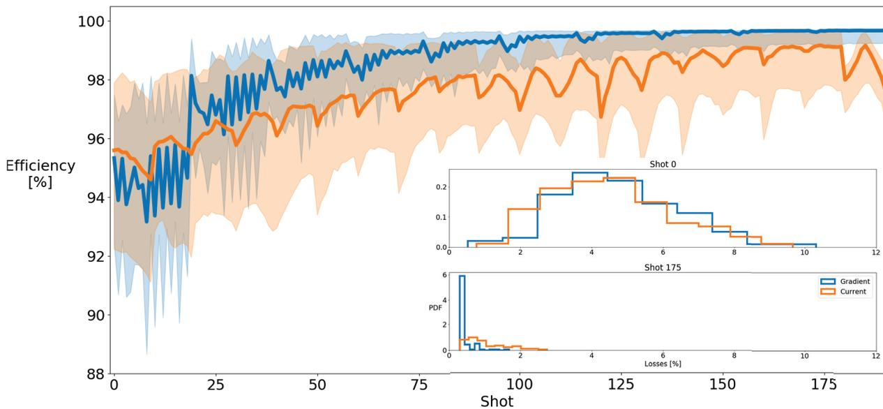
Figure 2: Simulations of the operational alignment procedure (orange) compared with a gradient descent algorithm (blue). The median and 90 % confidence interval are plotted from 200 error seeds randomly sampling initial anode positions from a Normal distribution with  $\sigma = 500 \mu\text{m}$ . Inset: distribution of extraction efficiency at shots 0 and 175.
