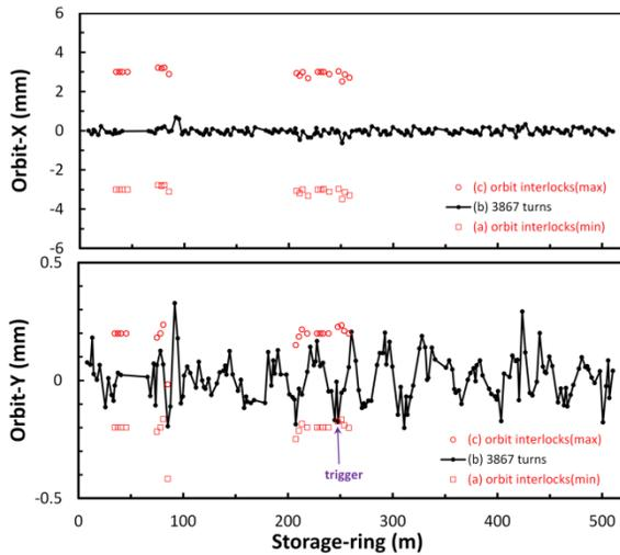
Figure 8: Orbit interlock triggered by a SD-165 current spike event.
