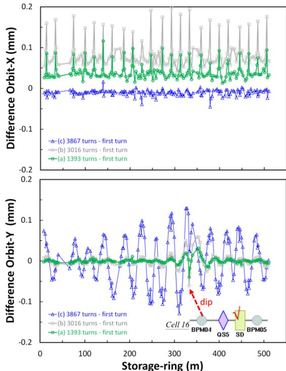
Figure 9: TBT-BPM Data analysis for a SD-165 current spike event.
