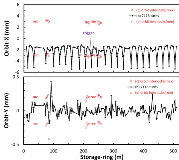
Figure 5: Orbit interlock triggered by an SRF trip.
