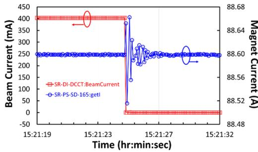
Figure 7: SD-165 magnet current record.
