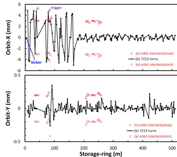
Figure 6: Orbit interlock triggered by kicker miss firing.
