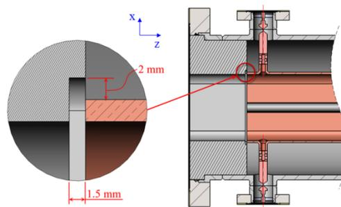
Figure 2: The detailed design of end plates projected to the x-z plane.
