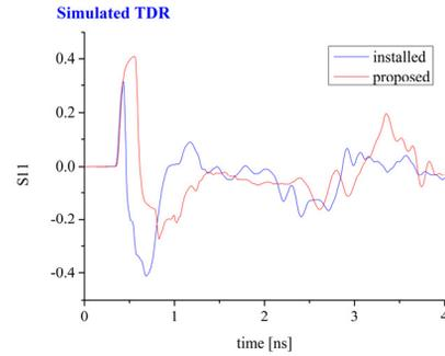
Figure 5: Simulated results of the TDR for the installed and proposed kicker designs. The time delay is manually adjusted for ease of comparison.
