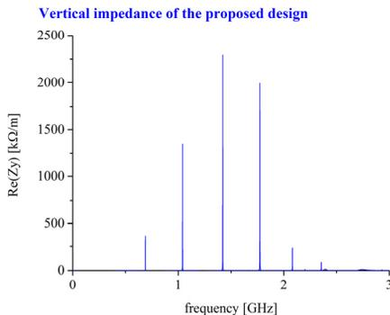
Figure 8: Simulated vertical beam impedance spectrum with a resolution of 0.2 MHz for the proposed kicker design.
