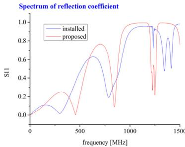
Figure 4: Simulated  $S_{11}$  reflection spectra for the installed and proposed kicker designs.
