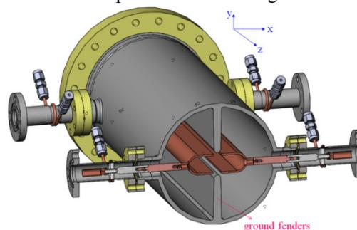
Figure 1: The mechanical design of the proposed horizontal kicker. Ground fenders are introduced to improve the impedance matching of TEM modes and reduce the loss factor as well.
