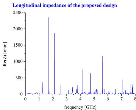
Figure 7: Simulated longitudinal beam impedance spectrum with a resolution of 0.2 MHz for the proposed kicker design.
