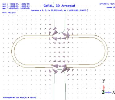
Figure 3: Simulated electric field patterns for the odd mode in the central region of the proposed kicker design.
