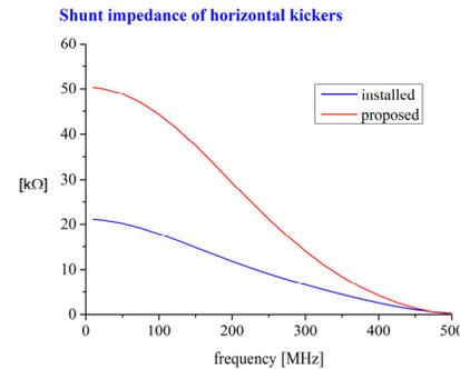
Figure 6: The transverse shunt impedances of the installed and proposed kicker designs. The shunt impedance of the proposed design is higher by a factor of 2.38.
