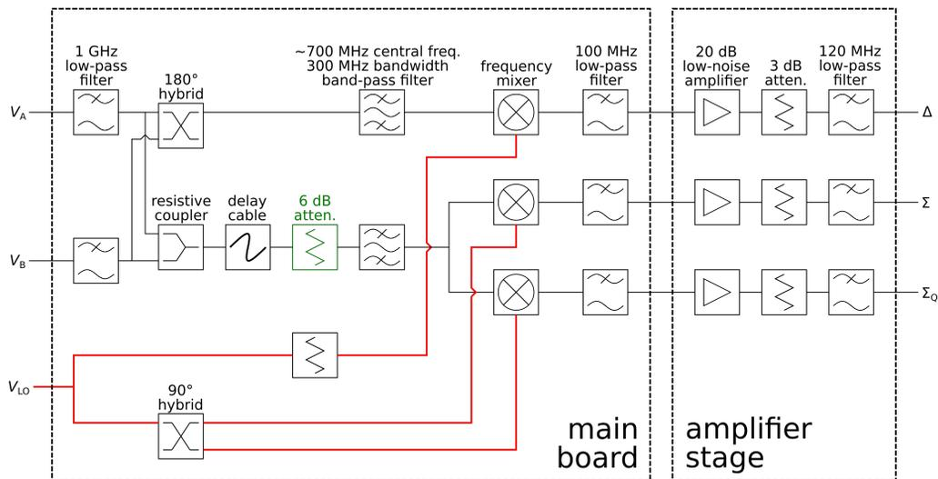
Figure 3: Schematic diagram illustrating the layout of the stripline processor modules. The local oscillator distribution is indicated in red.
