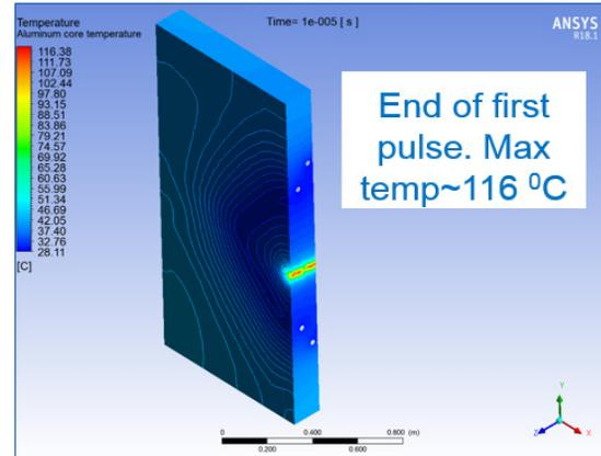
Figure 4: Temperature contours for the second aluminum core block after the first on-axis accident pulse.
