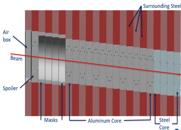
Figure 2: Cross-section of the absorber core with the red arrow indicating the central axis of the beam.
