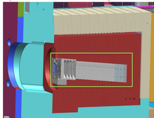
Figure 1: Cross-section of the absorber through the beam axis, the core is outlined by a green box.
