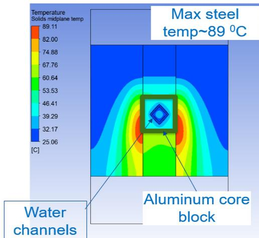
Figure 3: Temperature contours for the first aluminum core block (outlined by green box) and surrounding steel assembly. Maximum steel temperature is 89 °C.
