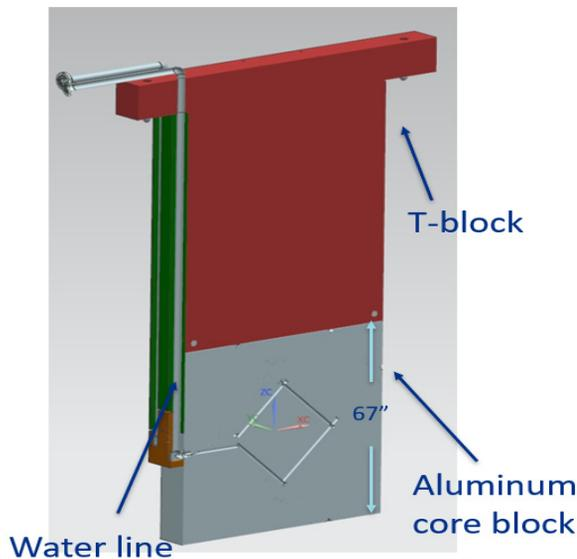
Figure 6: A standard T-block/aluminum core block assembly.
