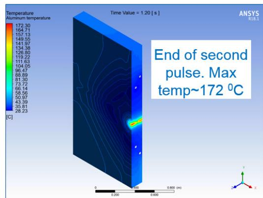
Figure 5: Temperature contours for the second aluminum core block after the second on-axis accident pulse.
