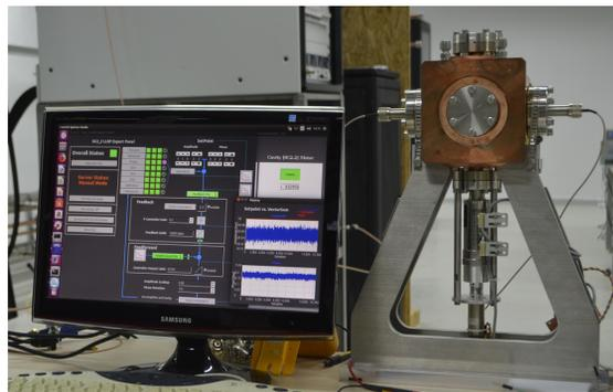
Figure 1: Controlling 1.3 GHz Buncher Cavity at TARLA.
