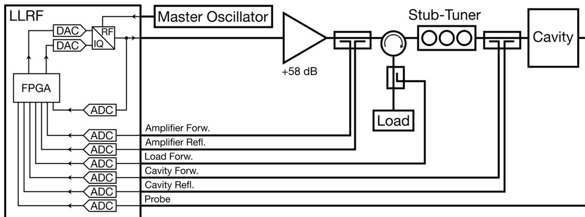
Figure 2: LLRF Setup for Commissioning at High Power.
