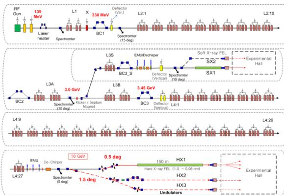
Figure 7: Schematic layout of PAL-XFEL.
