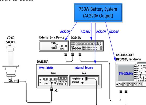
Figure 1: Test device for a stability measurement.
