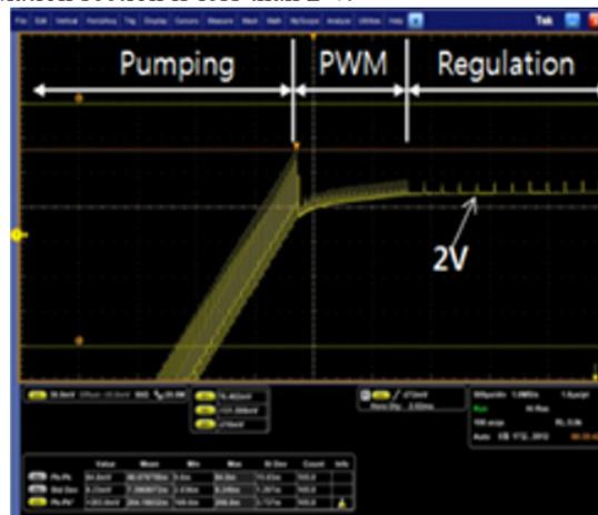
Figure 2: PFN charging voltage.
