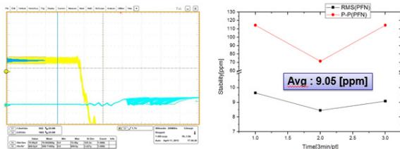
Figure 3: PFN voltage stability measurement.
