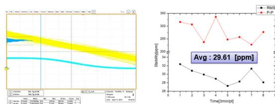
Figure 4: Beam voltage stability measurement.
