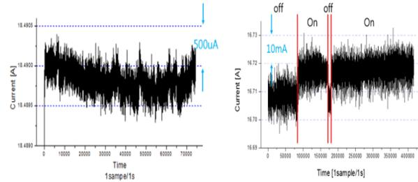
Figure 8: Current waveforms of MPS.
