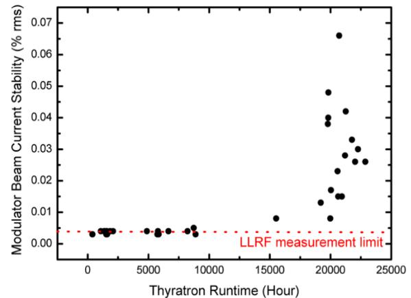
Figure 5: Modulator beam current stability according to the time aging at thyatron run-times.
