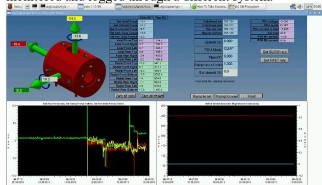
Figure 3: Solenoid control GUI, developed using EPICS EDM.
