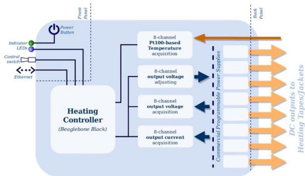
Figure 5: Block diagram of Baking Power Crates.
