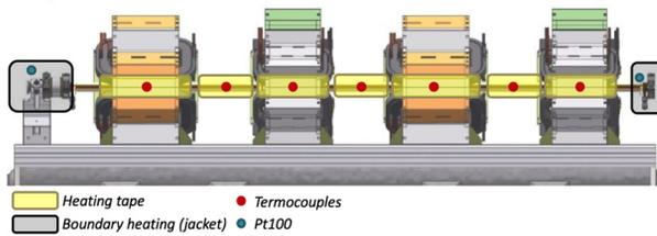
Figure 3: Experiment layout with thermocouples.
