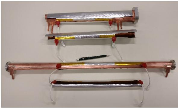
Figure 2: Tapes covering two different shapes of chamber along with the shape-memory after a heating process.
