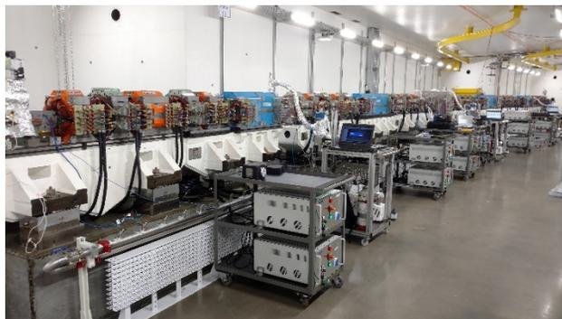
Figure 6: Bake-out system for one achromatic arc.
