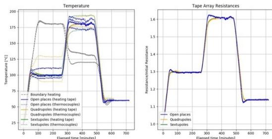
Figure 4: Temperature and tape resistances acquisitions during development of resistance heating control. Mean temperature readings reached an accuracy of  $\pm 8^\circ\text{C}$ .
