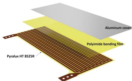
Figure 1: Developed ultra-thin heating tape.
