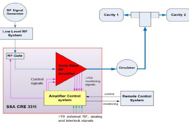
Figure 1: CLS booster solid-state amplifier RF block diagram [1].
