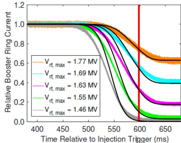
Figure 2: Comparison of measured booster current (coloured traces) with calculations based on quantum lifetime (black curves) for various cavity gap voltage with extraction time marked with red line [2].
