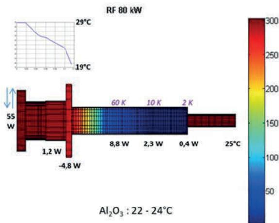
Figure 3: Temperature colour map (K) and resultant temperature (°C) and load (W) at particular sections of the coupler for 80 kW RF power. Coupler is tilted for plot convenience.
