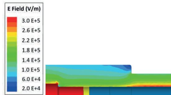
Figure 5: Electric field at 352.2 MHz @ 80 kW CW.
