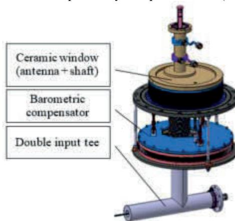
Figure 1: Main elements of the power coupler.
