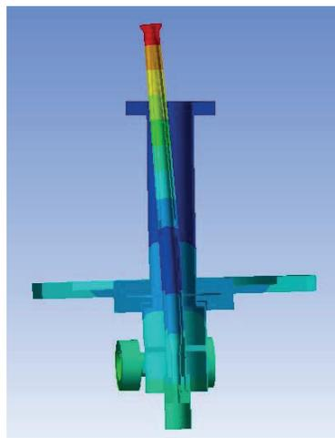
Figure 2: First vibration mode (antenna bending) at 72 Hz, cut view.
