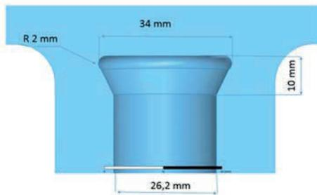
Figure 6: Design of the chosen antenna's tip.
