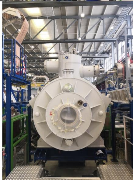
Figure 4: Top: Test bench overview. The three test benches (coloured blue, green, and white) can be seen. Bottom: short multiplert on test bench. On the left hand side are the power cable connection, on the right hand side the connection to the cryogenic jumper line.
