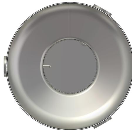
Figure 2: Cross section along the xy plane of the cavity. The angular coordinate of the HOM couplers was optimized and differs from the left to the right side of the cavity.
